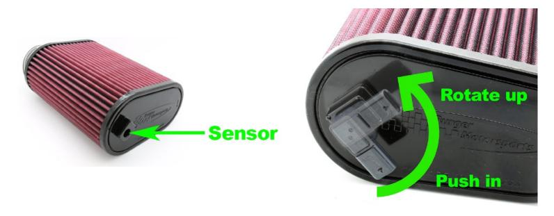
Loosely place the BMS intake pipe into the curved inlet pipe. Place the sensor into the BMS air filter. See photo below.
