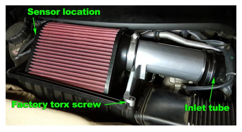
Now place the intake filter half in the lower half of the airbox shown in the photo above. Be careful with the delicate filter during this process.
