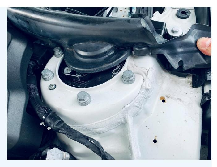
Push the rubber seals to one side so that you can gain access to the strut tower bolts.
