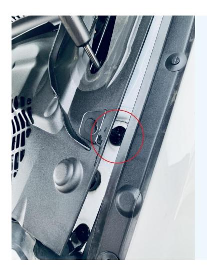
Pull out the cowl ensuring the cowl comes out of the push fit guide. Place the cowl(s) safely to one side.
