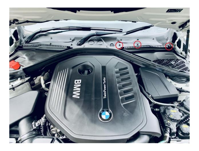
Loosen the screws on the right hand cowl. (Left hand side may also need to be loosened for 3 bolt version).
