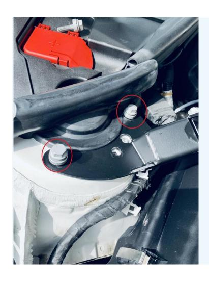
Screw the two outer bolts into the strut tower but do not fully tighten.
