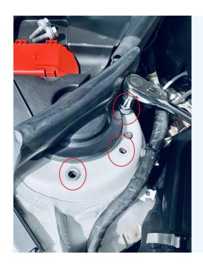
Using the 13mm socket loosen and remove the 3 bolts as per the image on each strut tower.
