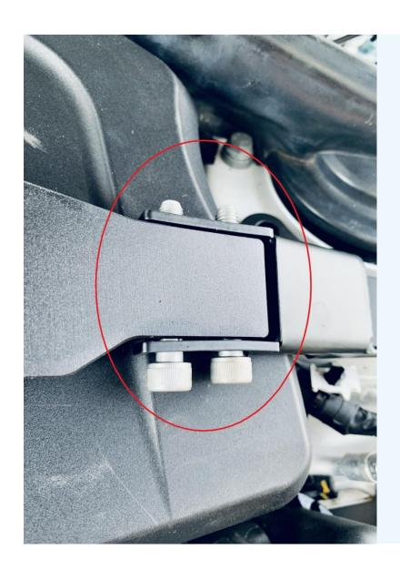
Using the Allen key and 12mm socket loosen and remove the 4 nuts located on each end of the strut brace (2 per side), however do not remove the bolts. Only use the Allen key to hold the bolt, do not turn).
