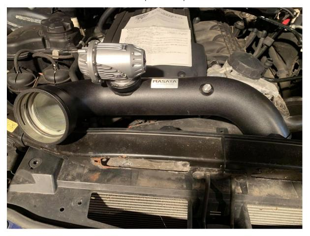
15. Transfer Chargepipe O-Ring from OEM Chargepipe to the Masata Chargepipe (Ensure it is seated in the Groove properly)
