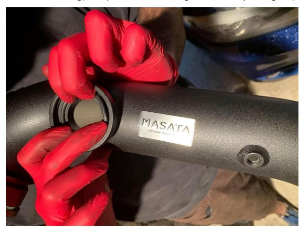
14. Install HKS BOV and secure it with C-Clip with a C-Clip Tool
