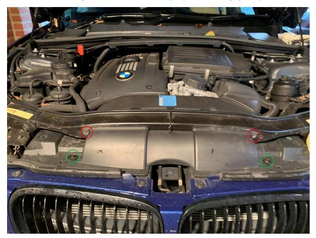
2. Remove Cowls(Green) and 2 x Lids (Red) - Unplug two bonnet sensor either side
