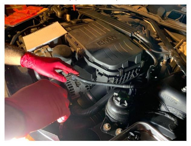
4. Loosen Front clamps connected to the airbox
