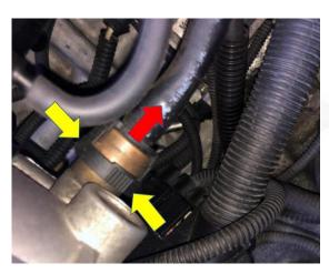
6. Remove the connector from the bottom of the throttle body by pressing in on the tab and pulling out. (This part can be tricky since it's underneath the manifold.) Sometimes it's easier to do this once the manifold is loosened up just be careful not to tug on the wires
