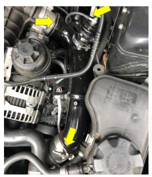
4. Remove the hard vacuum line by squeezing the tabs and pulling up.
