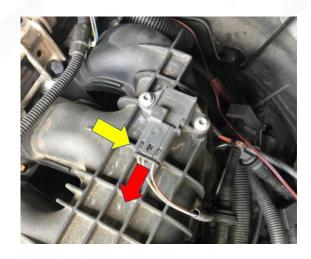
5. Remove the Vacuum line off the throttle body by pressing in the two tabs at the same time and pulling out.
