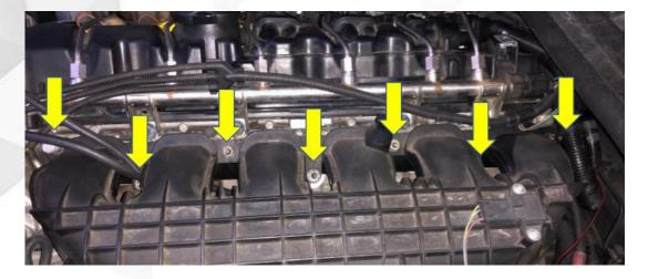
8. Carefully pull out the intake manifold making sure it doesn't get stuck on any wires. Now you are able to see the Low Pressure Steel Line and the Soft Line following it in the bottom right hand corner just under the starter.
