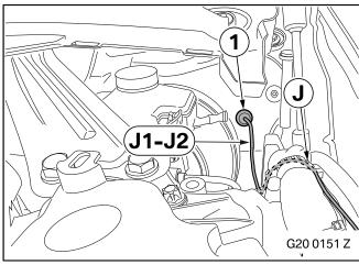
Route branches **J1-J2** from the engine bay into the footwell on the driver's side through the opening.
