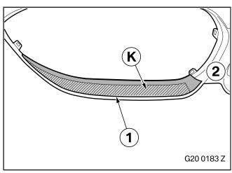
Pull the front section of the diffuser foil **K** (hatched area) up to the front edge (1) of the frame (2), affix it and run the blade over it.
