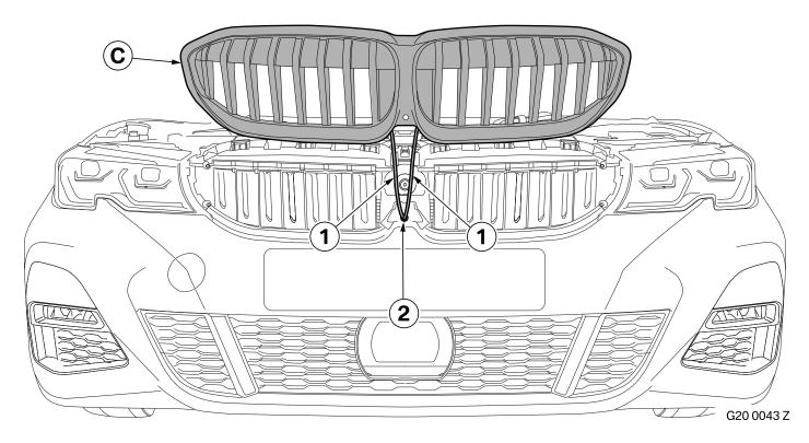
Thread the cables (1) from the front ornamental grille **C** through the openings (2) in the radiator louvre as shown above.
