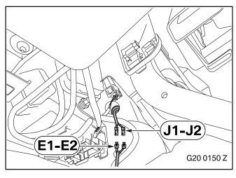
It must be ensured that the cables are not near movable parts while being routed. ◀
