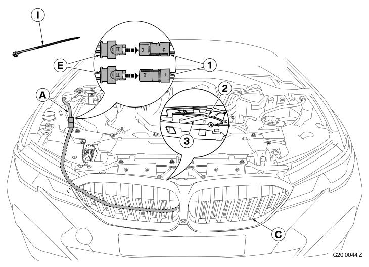
Route the retrofit wiring harness **A** along the standard wiring harness as far as possible and secure it with cable tie **I**. ◀
