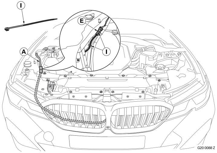
Secure plug  ${\bf E}$  to the standard wiring harness near the air filter as shown above using cable tie  ${\bf I}$ .
