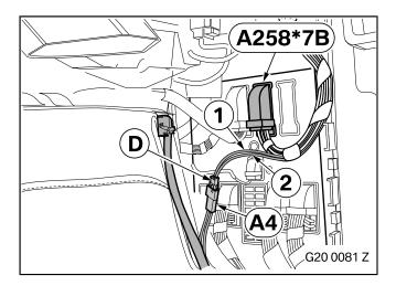
Disconnect the cables as follows from plug **A258\*7B**, WS 54-pin socket housing, and connect them to WB 2-pin socket housing **D**:
