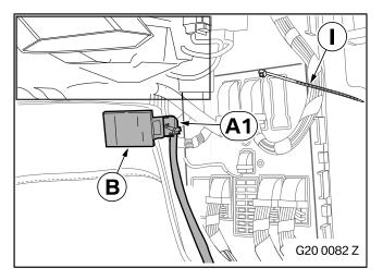
Connect branch **A1**, SW 12-pin socket housing, to CAN interface **B**.
