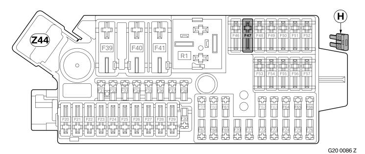
Place blade terminal fuse 3 A H into slot F47 of power distributor Z44.
