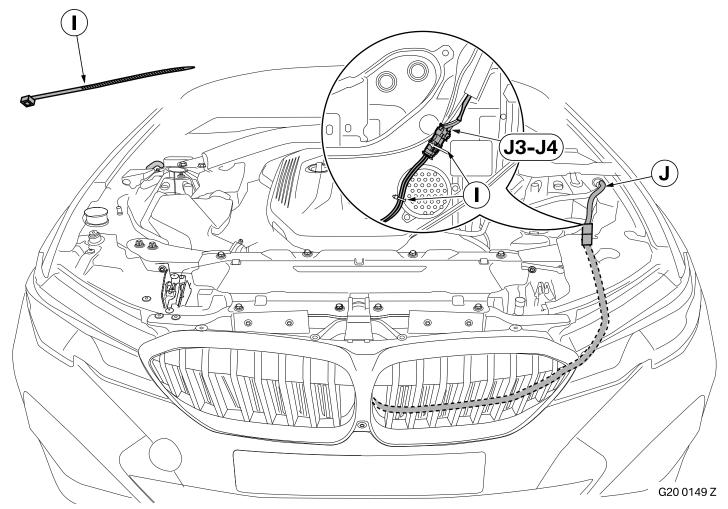
Secure plugs **J3-J4** to the standard wiring harness near the expansion tank as shown above using cable tie **I**.
