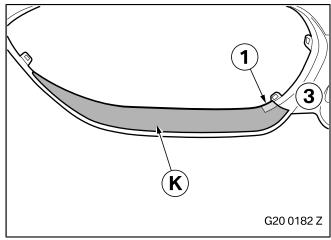
Pull the rear inner section of the diffuser foil  $\mathbf{K}$  (hatched area) up to the rear edge (1) of the frame (3), affix it and run the blade over it.
