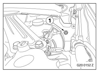
For PHEV cars or 48 V electrical system only Remove the recess (1) at the perforation using standard workshop equipment.
