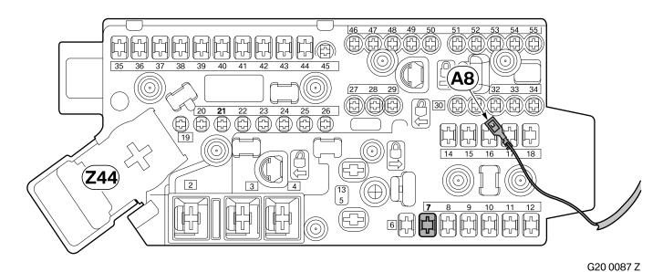
Connect branch A8, RT cable, to power distributor Z44 PIN 7.
