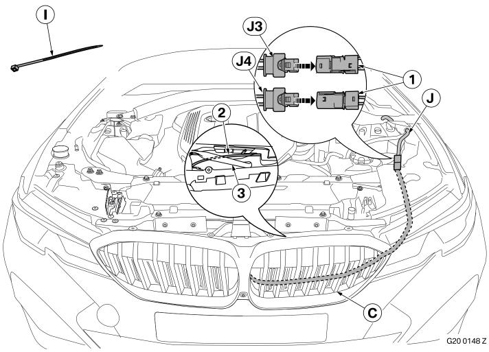
Route the cables (2) along the front ornamental grille **C** to the standard wiring harness below the V strut (3) and secure it with cable tie **I**.
