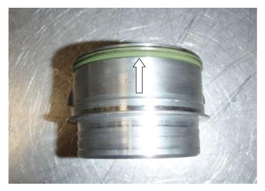
Drop the intercooler down and fit the male coupler into the intercooler, replace the clip and move up and down to ensure it locks in position. With the hose now in line move the intercooler up pushing the coupler into the hose, replace screws and tighten the intercooler. Position the JCS clip and tighten, replace the under tray and tighten all the screws. Installation is now complete!
