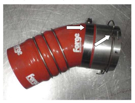
3. Carefully fit the coupler and hose in position taking care not to knock the clip out of position. Slide the clip up into the grooves of the coupler, move the hose/coupler up and down to lock into the grooves of the male coupler on the car. Push the intercooler up into its bolted position and rotate the hose around until it lines up with the inlet of the intercooler.
