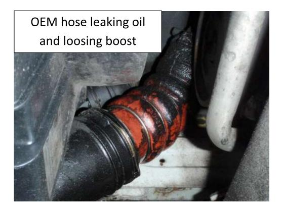
Tools Required: Flat headed screw driver T27 Torx driver 7mm hose clamp driver 8mm + 7mm socket Short extension and ¼ ratchet  Lift the car up either by jacking up and securing on axle stands or using a 2 or 4 post car lift. Remove the under tray, unclip the OEM hose. Undo the two screws holding the intercooler and drop down to allow access for removing the OEM hose.
