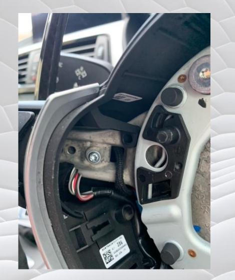
Once both paddles are fitted, re-fit the airbag and push back into the spring clips until its fully secured and clicks into place.
