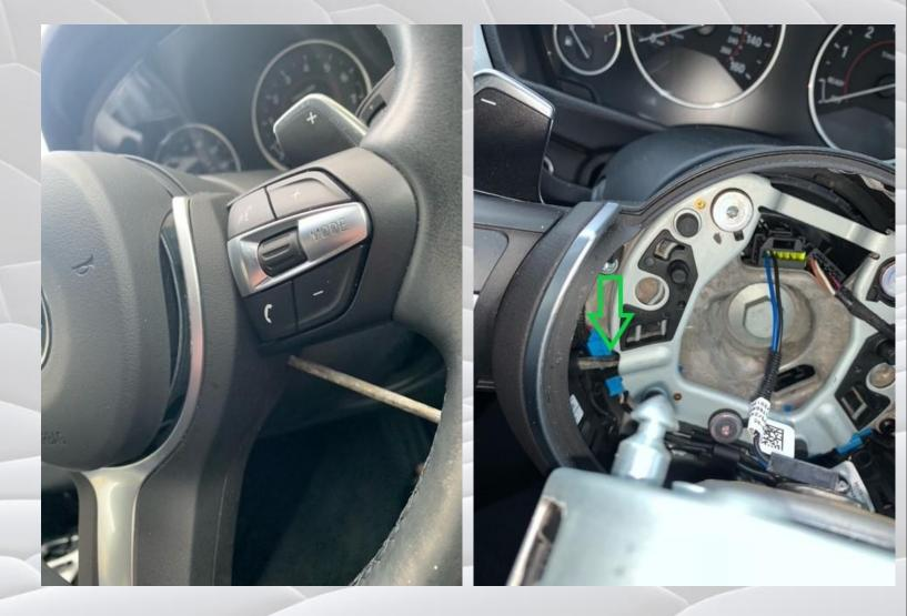
Either unplug the airbag or place safely on top of the steering column out of the way.
