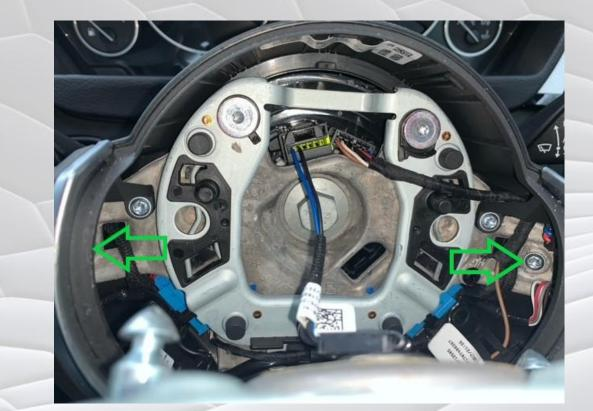
Using the small pick, push the pin out which holds the control/mount assembly together. The pin needs to be fully removed and set aside.
