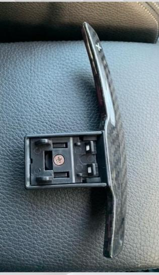
Re-assemble the control unit to the new paddle. And re-insert the pin. (reverse of step 4)
