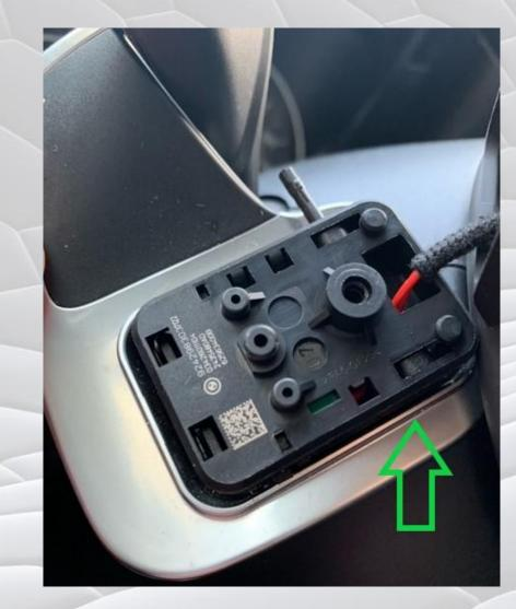
Using the new mounting equipment slide part no.2 into the paddle, and then slide part no.3 into this to complete the paddle and mounting assembly.
