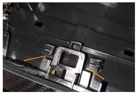
Reconnect the two cables and plug the trim strip to the dashboard.
