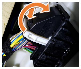
While When the clip is folded down, the plug is pressed out of the FEM a bit and can then be removed.
