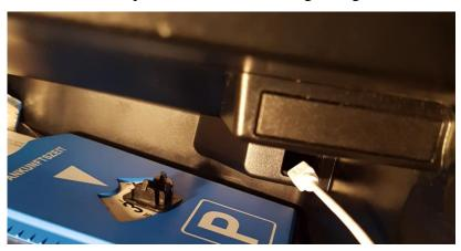
For LCI2 models, the small cover is omitted, the USB cable can alternatively be guided under the rubber mat through the opening.
