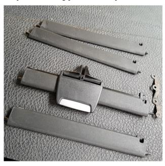
Disconnect any connector still attached to the air ducts and place it on the left side of the display frame:
