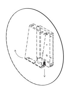
2: To seperate the sign face from the wall plate, pull the spring pin then rotate the bottoms apart.
