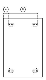
2: Measure from edge of board to edge of male cleat (A). Then measure from the outside of one male cleat to the outside of the other male cleat (B).
