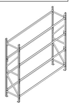
**Step 2** - Attach the remaining beams at the desired shelf height.
