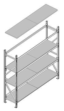
**Step 3** - Insert shelf panels so they sit flush on the beams. Start at the bottom and work your way up.
