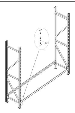
**Step 1** - Attach beams to the upright frames by slotting into the V channel and pushing down. Rubber mallet can be used if required. Insert locking clips to prevent the beam from being dislodged.
