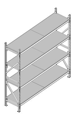
**Step 4** - Move unit into place and secure. It can be bolted to the floor using the included foot plates or secured with a tether (not included).
