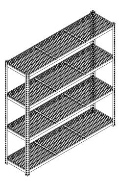
**Step 5** - Complete assembly and move unit into place. For added stability shelving should be anchored to a wall.
