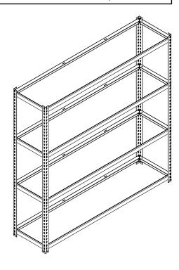
**Step 2** - Complete the frame by adding shelf levels at desired height.
