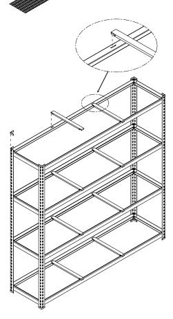
**Step 3** - Insert the shelf braces at each level and the plastic end caps for the top of the uprights
