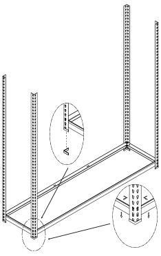
**Step 1** - Start by joining a long beam and a short beam to an upright. Be sure to have the flat edge of the beams facing up. Repeat for each upright and insert plastic end caps as shown.
