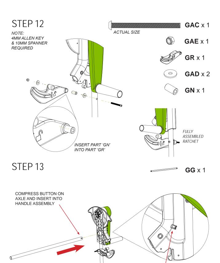
ENSURE SILVER BUTTON ON AXLE IS ENGAGED INSIDE THIS HOLE
