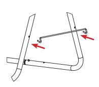
1. INSERT ENDS OF LEG BRACE INTO HOLE IN EACH LEG
