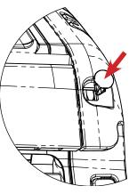
INSERT 4 SNAP CLIP INTO CORNER HOLES AS SHOWN IN DIAGRAM
