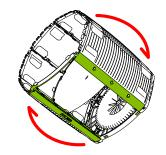
CAREFULLY FLIP BARREL AND REPEAT STEP 7 FOR OTHER END CAP
