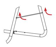
2. ROTATE LEG BRACE UP INTO HOLES SO THAT HORIZONTAL BAR SITS FLUSH AGAINST LEGS
