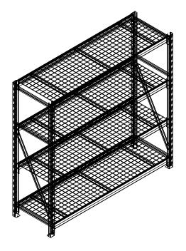
Step 5 - Complete assembly and move unit into place. For added stability shelving should be anchored to a wall.
