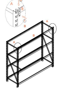
Step 2 - Finish beam assembly. Beam height is adjustable.
