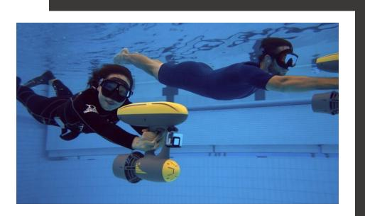
The propulsion system of an underwater scooter allows the rider to go swiftly through the water. It runs on batteries, and the runtime can vary from 30 minutes to over an hour depending on the battery capacity and the weight being towed. You will quickly find that operating an underwater scooter is easy to do:
