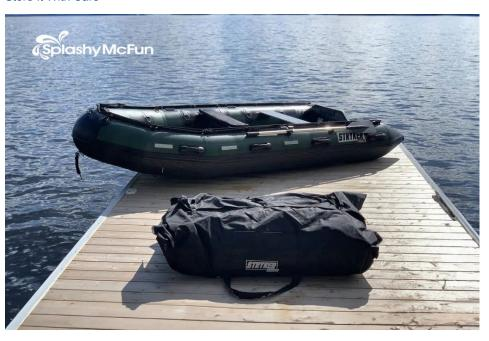
When the inflatable boat isn't in use, the best thing to do is store it partially inflated. Storing a completely deflated baot is riskier, as it is more susceptible to damage. But if you only have space for a completely deflated boat, ensure it's clean and dry before storing it.
