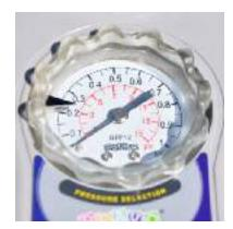
to read 3.2 PSI which is the operating pressure of your Sea Eagle. PSI is marked in red on the dial. Never turn the dial when the device is under pressure as this will immediately cause the instrument to break.
