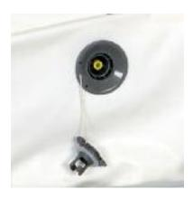
To deflate, remove the cap, press down on the valve stem and turn clockwise to lock into position. Release around 50-75% of the air from each chamber before fully deflating. Excess air can be pushed out as you rollup the boat.
