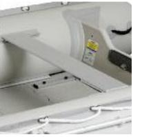
Aluminum Bench Seat Transom Boats come equipped with a bench seat and two sets of fabric beads (back and front) to secure the bench seat to. Your boat should be around 50% inflated before installing the bench seat. Please note the second bench seat is sold separately.
