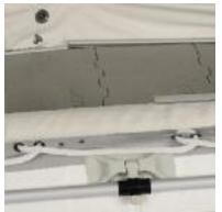
Once deflated, loosen the side stringers with your foot and remove both the stringers and floorboards. You do not need to remove the supports on the FB-2 & FB-4 floorboard pieces. If you have a drop stitch floor, you can deflate it and roll it up with the hull.
