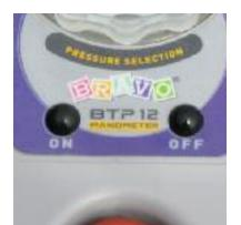
Press the ON button to begin inflation. The pump operates in two stages which can be identified by the noise of the turbine at the start, followed by the piston. The pump automatically stops once the pressure is reached.
