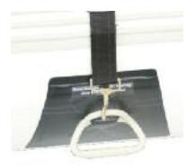
Tie the two rear straps to the back of the boat and then clip the front strap of the canopy to the rope lacing. Keep in mind to tighten the canopy so that it is level and so that it fits tightly on your Sea Eagle.
