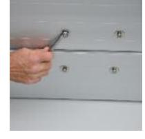
Use the screwdriver at the top of the bolt to hold it in place and at the same time use the crescent wrench on the nuts on the bottom to tighten the bolts for the seat mount.
