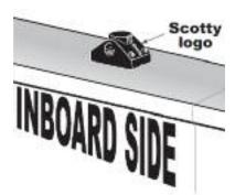
To install the mount, place it over the desired area and drill a 1 3/8" through the fittings at each end of the mount. Be sure the "logo" on the mount reads upright when looking from inboard before securing the mount with the provided hardware.
