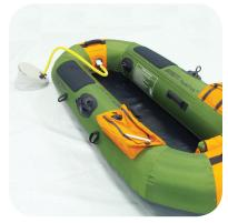
Insert hose into the second chamber and inflate until firm. This is the main flotation chamber. Most of the wrinkles should be out of the cover.
