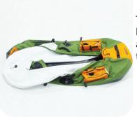
To inspect the air bladder, deflate the boat and pull the bladder out the zipper opening.
