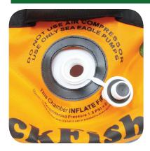
Unscrew the valves from the bases. Most of the air will release immediately. Remaining air will push out as the boat is folded.
