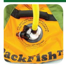
Insert hose into the first chamber valve and pump until firm. This is the safety chamber.
