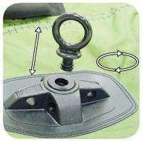
Screw the oarlock rings into the bases.
