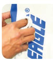
Thoroughly clean and dry the area surrounding the leak. Circle the leak to make locating it easier throughout the repair process.
