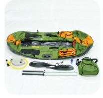
Select a flat, hazard free area to unfold the boat. Locate the air valves and oarlock rings.
