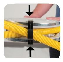
Unravel the hose and push down on the top & bottom of the pump to release the black clip.
