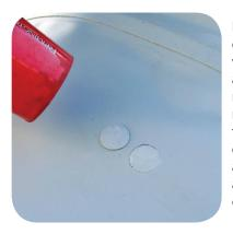
If you have access to electricity, heat the glue with a hair dryer then apply the patch. This method produces the best results. Mate the patch to the board and smooth down until the patch adheres. Do not inflate, allow at least 24 hours to cure before inflating.
