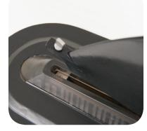
Line the screw up with the plate and push the skeg down. A little force may be needed to get it in place.
