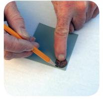
Trace the outline of a penny on the patch material and cut using scissors. Trace the outline of the penny on the SUP. Coat the patch and SUP with the repair kit glue.
