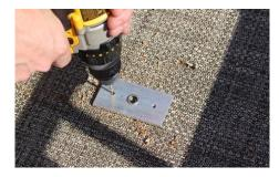
Step 8: Remove the plates and enlarge the holes to 5/16".
