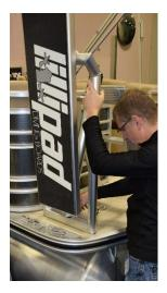
**STEP 1.**Position the frame over the frame mounting hole and secure it to the plate below using an eye bolt.
