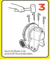
Check product anchorage during use and re-secure if needed.
