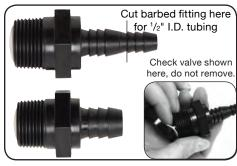
2. <sup>3</sup>/<sub>4</sub>" MPT barbed check valve is designed to be used with 1/2" or 3/8" I.D. tubing. Use larger barbed fitting for 5/8" ID tubing
