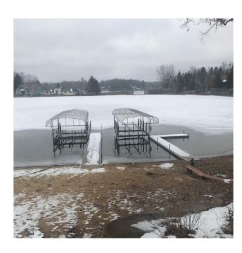
This dock bubbler system uses 2-6 compressor with self-weighted air diffusers to create an air flow up to 6.5 cfm. 3/8" quick sink tubing allows for quick and simple installation.
