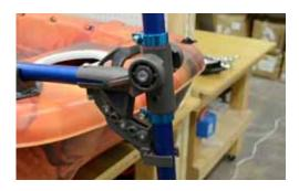
If you have foot pedal steering on your kayak, you can run your foot pedal lines to the Bixpy vertical pipe "wing" instead of using the Bixpy steering handle.
