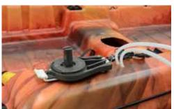
Run your left and right lines through the tubing until they come out from the back near your vertical pipe.
