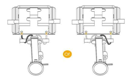
Step 3: Insert handle base into slot and thread axle through jack and handle. Lock in place with circlip
