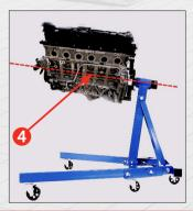
Lock mounting plate in position before attaching the engine.
