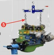
Use correct model for intended applications. An engines length, width and weight should never exceed the engine stands foot print dimensions or weight specifications.
