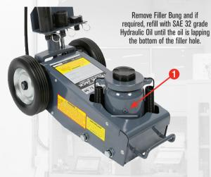
Regularly lubricate the Air motor. Lubrication of the Air motor is essential for smooth operation while raising a vehicle.
