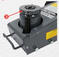
Storage in the fully lowered position ensures the lift ram assembly and pump piston is sealed from exposure to weather fluctuations and keeps the hydraulic ram and pump seals in a relaxed condition ready to work when required.
