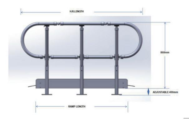
1. Connect the ramp to the support legs. Use the supplied M7\*16 screws, spring washers, and gaskets to secure the sliders inside the support legs
