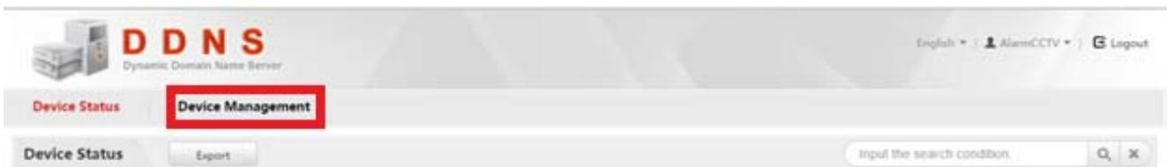
10. Select “Add” and enter the “Device Serial No.” which was the nine digit number you copied from step 7. Enter the “Device Domain” name which you made in step 5. Enter the forwarded “HTTP” port (default port is 80) into the “HTTP Port” section.
