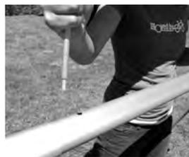
The banner poles drop into any of the 3 holes in the fully extended inner main tube.
