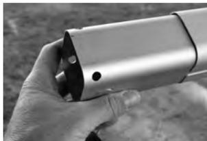
Extend the rack until the push button locks in place at its fully extended position.
