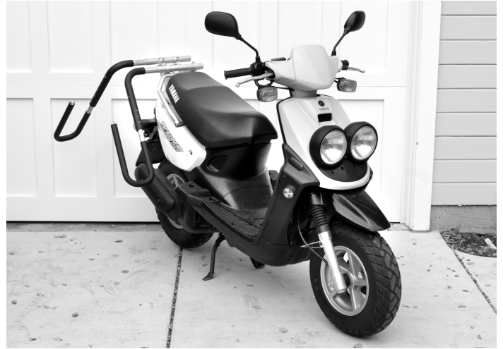
When rack bars are mounted together on a rear rack, they are recommended for short boards up to 7-8' in length
