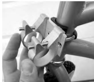
5. Slide the mounted tube into the tube clamps.
