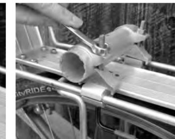
1. Loosen the hardware enough to slip the clamps over the rack rails.
