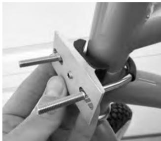
4. Replace the tube clamps on the U-bolt.
