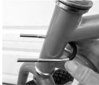
3. Place the saddle on the head tube. Loosen the set screw. Leave the rubber cover on to protect paint, or remove it for better clamping.
