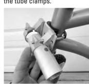
2. Loop the U-bolt around your head tube. There are three sizes. Use the smallest that fits.
