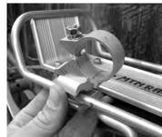
1. Loosen the hardware enough to slip the clamps over the rack rails.
