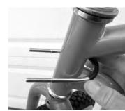
**4.** Replace the tube clamps on the U-bolt.
