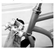
Place the saddle on the head tube. Loosen the set screw. Leave the rubber cover on to protect paint, or remove it for better clamping.
