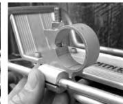
2. Partially tighten the hardware to keep the tube clamp in place.
