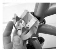
**6.** Reinstall the washers and nuts and tighten with a 10mm wrench.
