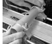
**4.** Center and align the mounted tube.
