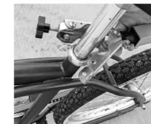
Position clamp around seatpost
