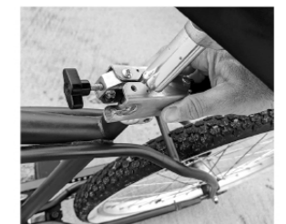
Close clamp onto seatpost
