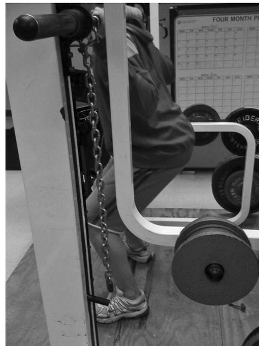
**Figure 4.** Side view of isometric squat test set up with heels positioned over marker 1, feet shoulder width apart and Knee joint angle standardized to  $135^{\circ} \pm 5^{\circ}$ .
