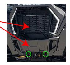
Step 2: Mount included bracket above the winch mount with the included 1/2 inch nuts and bolts. Once the included bracket is installed. Mount the plastic winch cover back on to the machine.
