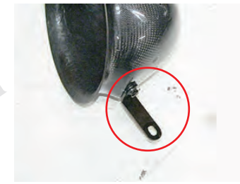
6. Attach the brace to the carbon introduction duct with bolt A.
