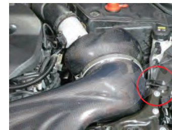
15. Secure the brace to the rubber damper using nut (M6).
