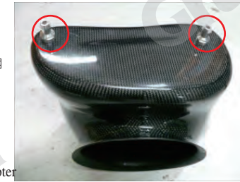
9. Attach the aluminum stud to the chamber box using bolt B.
