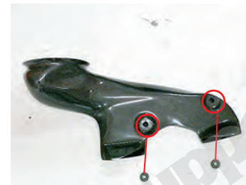
5. Attach the grommets removed in step 2 to the carbon introduction duct.
