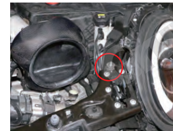
12. Install the rubber damper on the body.
