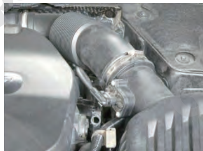
3. Disconnect the air mass sensor coupler and loosen the hose band.
