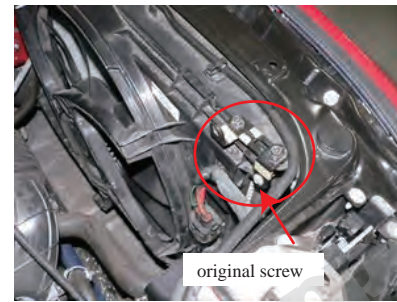
7.Mount assembled brace in step 6 using factory screw to location shown here.
