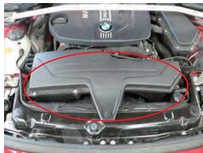
1.Remove the air box assembly.
