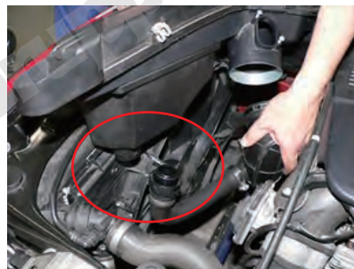
2.Remove MAF (Mass Air) coupler. Loosen coupler and suction hose band. Remove air hose located on the bottom side of the case
