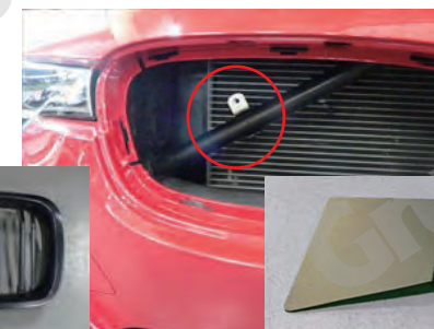
17.Place the "U" bracket on the back of the bar running diagonally in front of the radiator and attach to the induction plate using bolt B from the front side.
