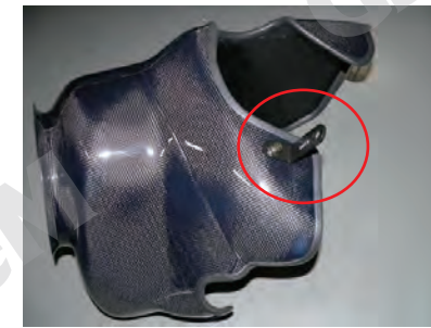
8.Using bolt A attach brace (0076B) to the filter case. (Using bolt A)
