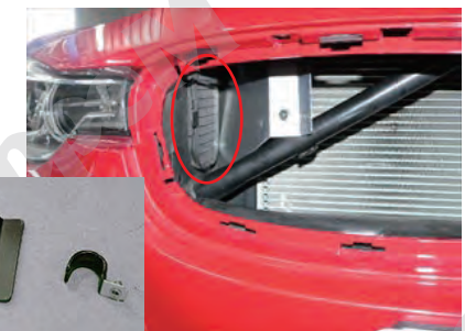
18.Adjust the induction grille so that fits the original inlet. Next, re-install the grille. Please see the attach picture for details.
