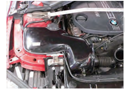
9.Install in engine bay while being careful to avoid air duct guide, engine harness and hood release cable.
