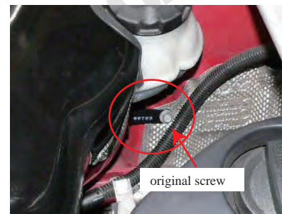
10.Mount the air filter case to the body as shown using original screw.
