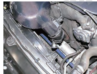
13.Attach the suction pipe to the chamber case. NOTE – be sure not to over tighten when installing, this could damage or break intake casing
