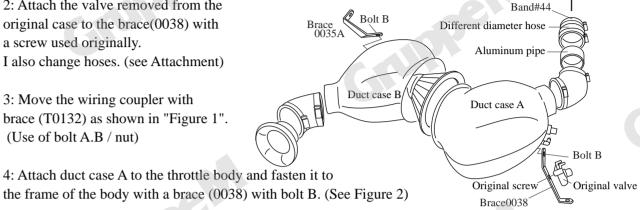
5: Hold the filter in the duct case B and assemble it with a band. At the same time fasten the body and duct case with braces (0035A). Use bolt B (see Figure 3)
