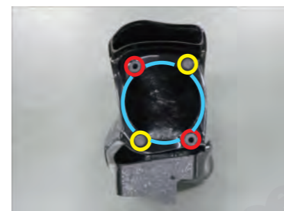
7. Attach the grommet and sponge tape. Red : O-ring grommet Yellow : Solid grommet Blue : Sponge tape (thick) Cut and attach the sponge tape.
