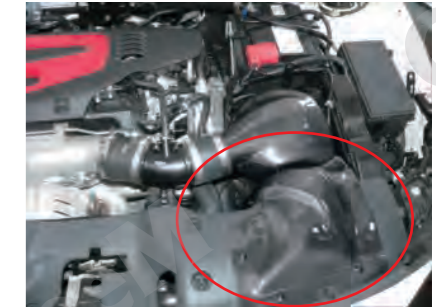
30. Install the front introduction duct as circled in red.
