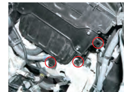
6. Disconnect the three connectors of circled in red. The wiring interferes with other work, route it around the battery.
