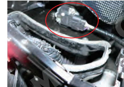
33. Attach the wiring coupler to the air mass sensor.
