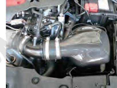
29. Re-install the intake chamber assembly again and tighten the hose band.
