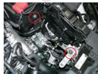
10. Attach the rubber stud bolts to the location circled in red
