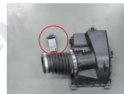
2. Remove the air mass sensor from the air cleaner box.
