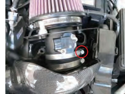
28. Check that the hose band has not slipped off and retighten the band.
