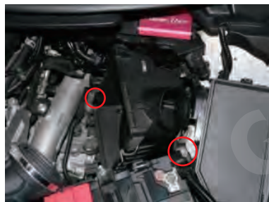
5, Remove 2 bolts and take out the bottom of the box.
