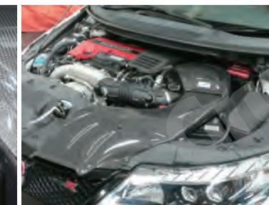
24, Please close the hood slowly and check the clearance for interference with the introduction duct. Adjust accordingly.
