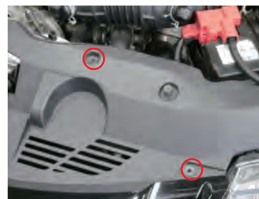
17, Remove the clip on the radiator cover and insert the wellnut from above into the hole.
