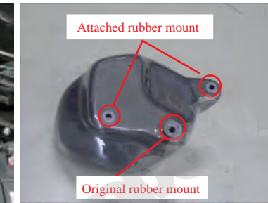
11, Attach the rubber mount to the carbon box.
