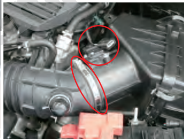
2, Disconnect the sensor connector and loosen the suction hose band.
