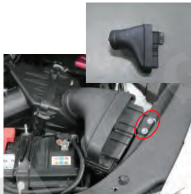
1, Remove two bolts and remove the introduction duct.
