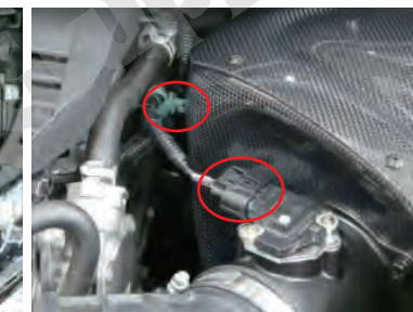
23, OE connect the air mass sensor. Push the wire clip into the carbon box and fasten it.
