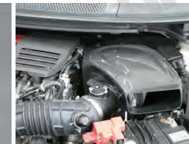
16, Place a carbon box. Insert the mounting rubber at the bottom of the box. Check that the box is secure in the protrusion of the bracket.
