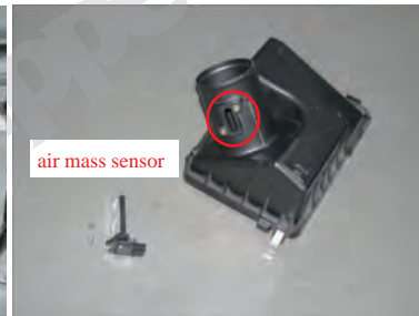
4, Remove the air mass sensor from the top of the box.
