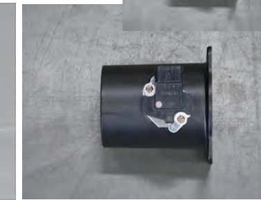
12, Install the conversion plate with bolt E to the sensor adapter. Fit the air mass sensor with the M4 spacer, and attach the air mass sensor with the bolt F.
