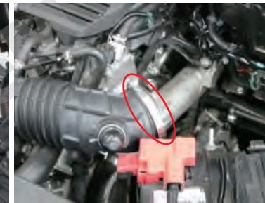
10, Replace the hose band with the included hose band. (The original hose has bumps. Using the attached hose band, press the protrusion down.)
