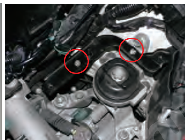
7, Remove the filter box bracket.
