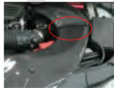
21, Insert the carbon introduction duct into the carbon box. Be careful not to peel off or damage the cushion tape.
