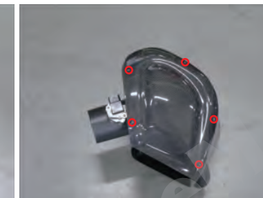
15, Install the carbon box cover. (Using the bolt that was assembled)
