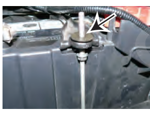
12. The installed bracket should be mounted in the following order on the battery j-bolt: upside down OE nut -> washer -> battery hold down -> brace -> nut.
