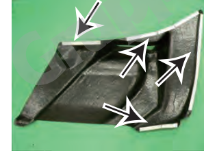
23. Attach double-sided tape to the back side of the air duct as shown in the picture.
