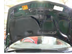
22. Re-install the cut part of the hood insulator and secure with OE clips. The center is secured together with the carbon air duct.
