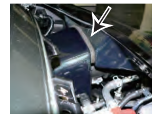
32. Close the hood/bonnet once to confirm the filter case and the induction duct is connected properly and the brace is secure.
