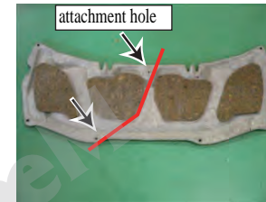
19. Cut the hood insulator in half as indicated by the red line. NOTE - For LHD applications, cut opposite as shown.
