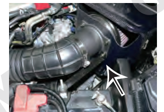
31. Mount the brace to the filter case assembly as shown.
