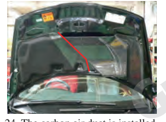
24. The carbon air duct is installed using double-sided tape. The edge of the carbon air duct will slightly overlap the cut hood insulator as shown in the picture.
