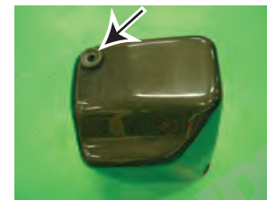
28. Install the rubber mount removed from the OE air box to the filter case as shown.
