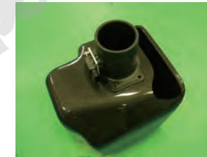
26. Attach the MAF adapter to the filter with the MAF connector in the downward position. Secure with bolt A.
