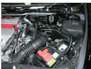
8. Loosen the hose clamp then remove the upper OE filter assembly followed by lower assembly and air duct.
