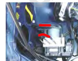
A protection tube is put on ABS piping of the red line mark.
