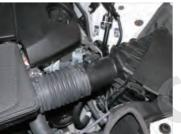
7. Take out the opposite box as well. 8. Remove the air mass sensor.
