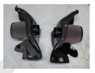
12. Attach the filter to the funnel adapter.
