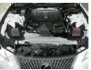
14. Place the carbon case assembly in the engine compartment and attach it to the suction hose.
