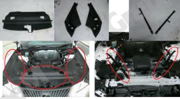
1. Remove the clip and remove the engine compartment panels indicated by the red circles.
