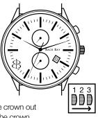
Setting the date: Pull the crown out to the 2nd position. Turn the crown counter-clockwise to set the date. After the date has been set, push the crown back to position 1.
