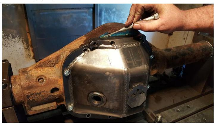
• Remove the cover and using the bottom plate mark the cut line on the housing by aligning it to the previous mark and scribing a line. **Important...** this line is only a guide. Machine the housing to a point where accurate measurements can be taken.
