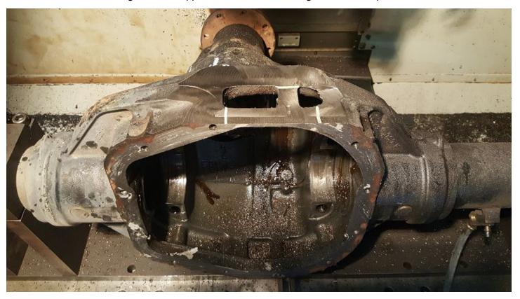
• Using a cut off wheel or saw remove the supports to ensure they do not break off while machining.
