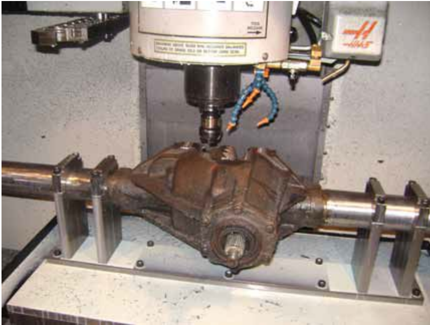
Fig.2 (Ring Gear installed to confirm dimensions)
