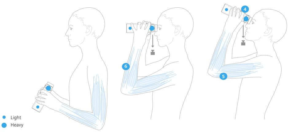
The center of gravity of the glass on the ZEISS VICTORY SF was consciously moved towards the eyepiece for improved ergonomics and user comfort. 4 Thanks to the ErgoBalance concept, the
