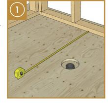
Perform a final floor and wall measurement check to ensure all walls are square and make any adjustments required BEFORE installing your shower system. Remove and clean up any construction dust, dirt, and debris from the shower install area. [fig. 1]
