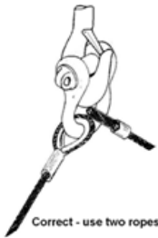
Correct - use two ropes with eyes
